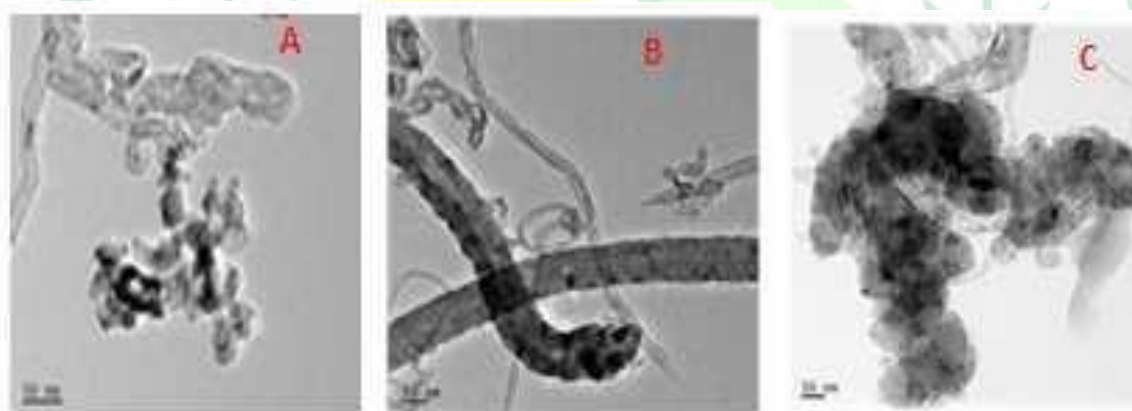
Fig. 4.1.3. TEM images of (A) MWCNTs, (B) MWCNT-CH=CH 2 , and (C) MWCNT-IIP
