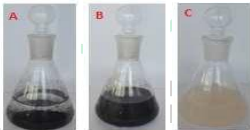
Fig. 4.1.6. Photographs of (A) MWCNTs, (B) MWCNT-CH=CH 2 , and (C) MWCNT-IIP dispersed in water
